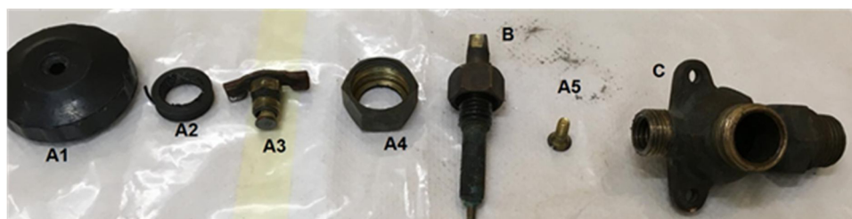
Fig. 10. Contaminated piece 1 disassembled into parts: handwheel (A1), packing (A2), wing bolt screw (A3), nut (A4), screw (A5), stem (B) and valve housing (C).
